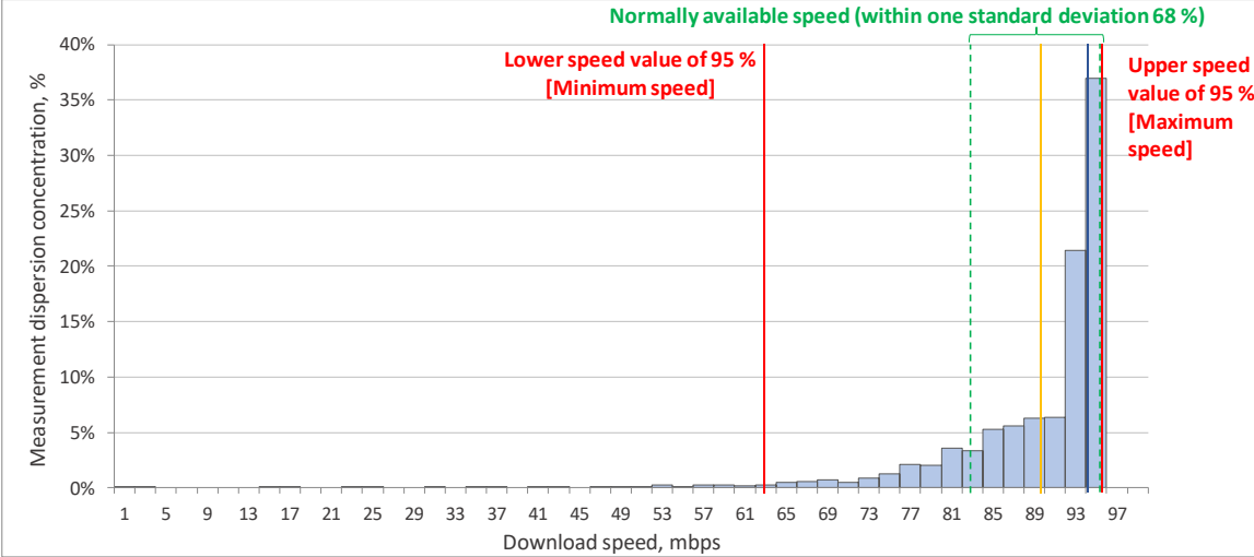
Fig. 9. Example of broadband Internet download connection speed measurement data concentration in a fixed network (FTTH 100 Mbps).
