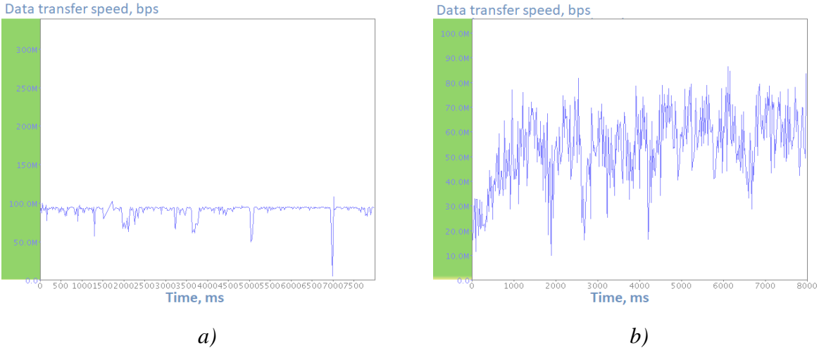
Fig. 6. Example of experimental measurement of changes in download connection speed: a) in fixed FTTH (100 Mbps) network; and b) mobile 4G network.
