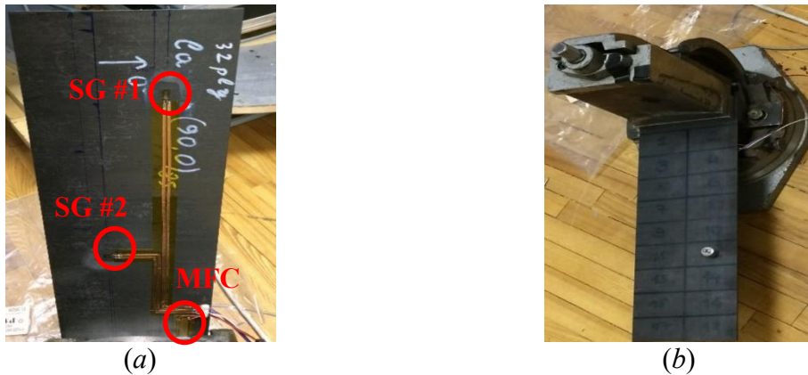
Fig. 5.4. Cantilevered CFRP plate: (a) photo; (b) partition into zones and application of mass.
