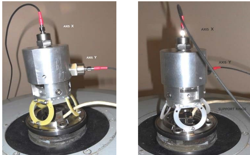
Fig. 5.1. Arrangement of accelerometers that measure the vibration accelerations of the detector unit on the ring supports from the Composite G-Etronax (left) and CESTILENE HD 1000 (right) material.
