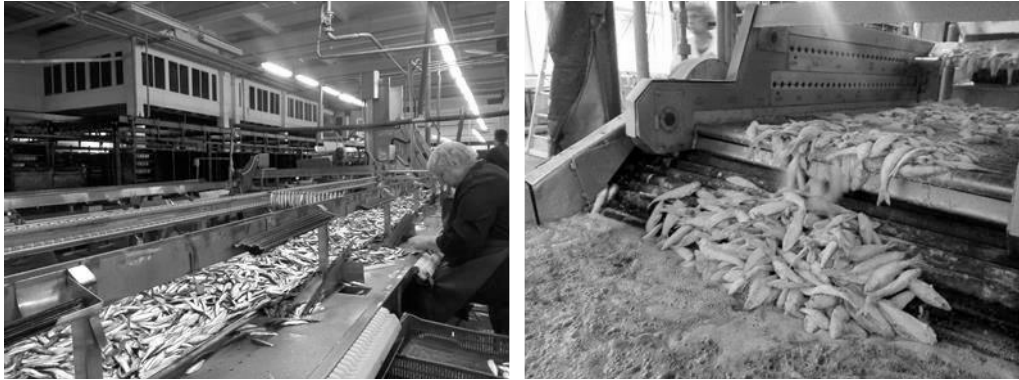
Fig. 2.17. The analyzed fish processing company: fish grading (on the left), fish roasting (on the right).
