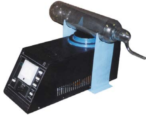
Fig. 2. Small-size generator of pulse currents for processing powder materials.
