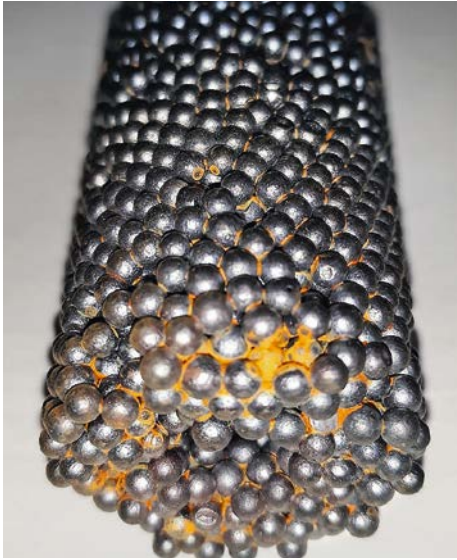
Minispheres after compaction.
