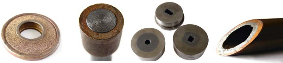
Powder-like bronze before and after processing by a pulsed electromagnetic field.
