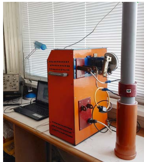
Fig. 4. Experimental device for moving ferromagnetic powders by the pulsed electromagnetic field, providing lifting of about 1 kg of powder as high as 3 m.
