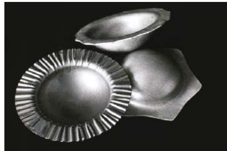
Fig. 5. Flat electromagnetic punching.
