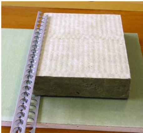
Punched profiles used for the production of inner wall panels.
