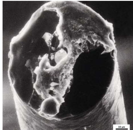
Microstructure W-B fiber.
