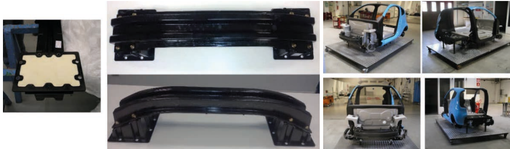
Fig. 3.10. EVolution front bumper crossmember demonstrator prototype and the technological mock-up with integrated demonstrators.
