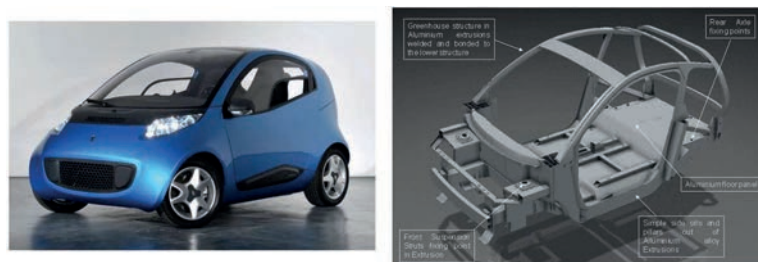
Fig. 3.9. Nido concept (left) and Nido BiW (right).
