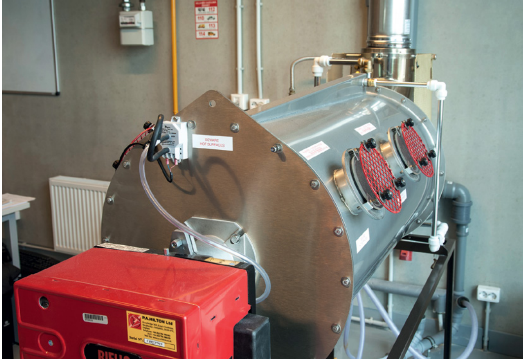
Combustion Laboratory unit C492 Gas Burner Fitted.
