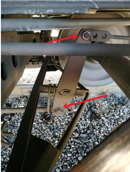
Fig. 1.8. Vertical lever of the brake lever mechanism of a freight car (arrows denote mounting points).
