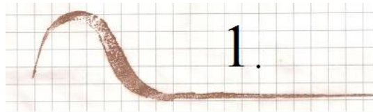
Fig. 5.1. Representation of the characteristic wear of the running surface of a freight train wheel, found in “Latvijas dzelzceļš” network.
