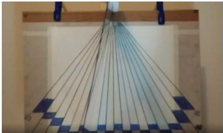
Fig.6.11 Motion of the pendulum oscillating about the mean position.
