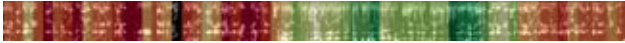
Figure 6: Segmentation of audio sample for speaker diarization task for 2 male speakers. Red frames are furthest away from speaker feature embedding vector and green frames are closest thus identifying target speaker 1 .
