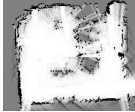
Fig. 11. Map generated from LIDAR point cloud on 2D plane from mobile robot platform.
