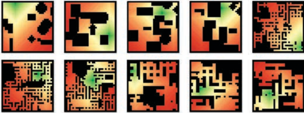
Figure 21: Examples of synthetic maps generated by OccupancyMapGenerator and cell values to reach the positive terminal state (Green - the highest value, Red - the lowest value).
