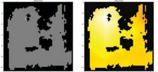
Fig. 12. Discretized map from LIDAR point cloud on 2D plane on the left. The map of values of states after passing through UNet-RNN-Skip model on the right.
