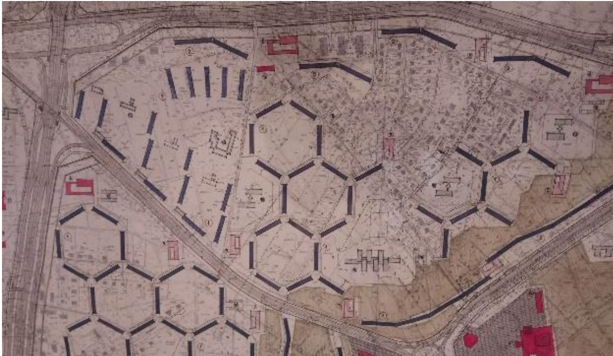
Fig. 3.3. Fragment of Purvciems large-scale housing estate detailed plan (showing the combination of parallel blades, surround-type structures which form hexagonal courtyards and semi-closed forms) [262].
