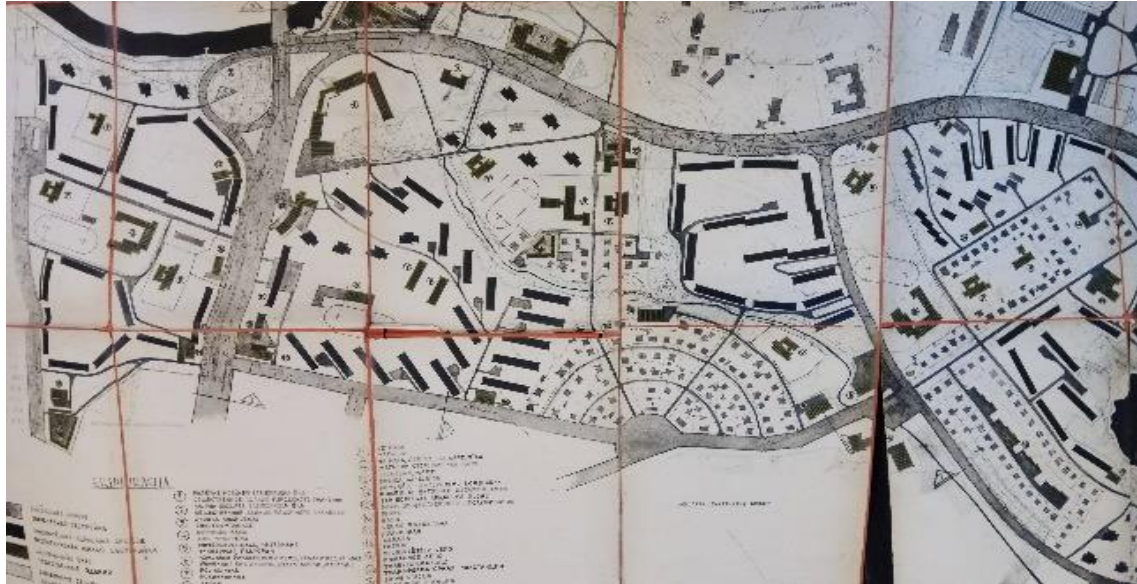
Fig. 3.1. Fragment of the detailed plan Lielā Jugla large-scale housing estate (showing the combination of parallel blades, high-rise towers, surround-type structures and semi-closed forms) [262].
