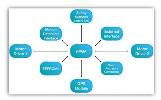
Fig. 5.2. FPGA's peripherals block diagram.
