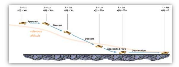
Fig. A.2. Reference landing manoeuvre altitude against vehicle's manoeuvre position, graphical animation.
