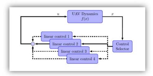
Fig. 2.3. Schematic of a gain scheduled scheme for UAV control [3].
