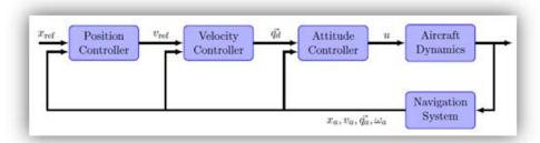
Fig. 2.1. Successive loop-closure control architecture [2].
