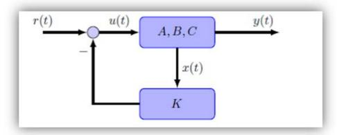
Fig. 2.2. Full-state feedback controller [2].
