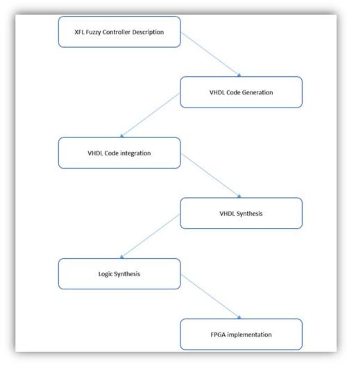
Fig. 4.1. Proposed design flow.
