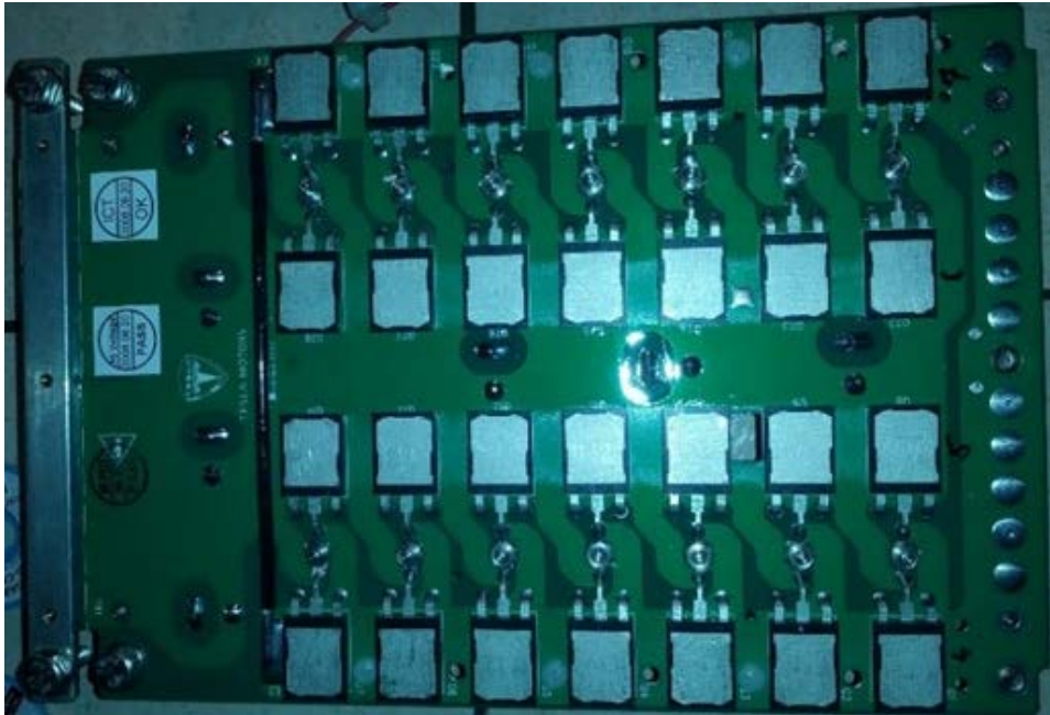
Figure 3.8: TESLA Model S half-bridge inverter power PCB.
