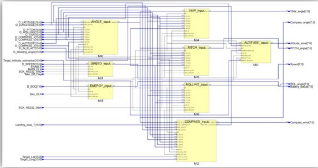
Figure 6.65: RTL view, the outcome of the “Digital_Processing” VHDL component algorithm’s synthesis.
