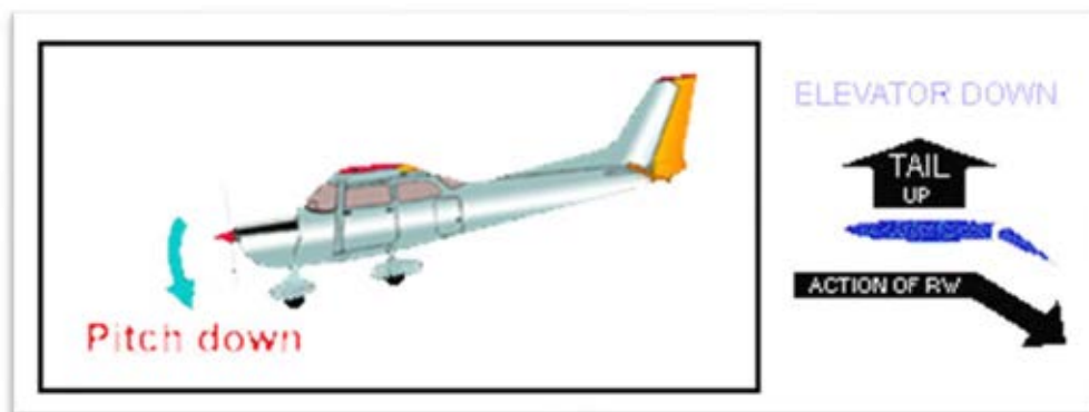
Figure 6.25: graphical representation of the effect of the elevator action on the vehicle's pitch angle.
