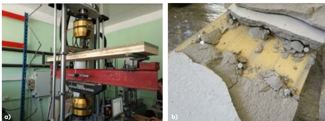
Fig. 1. Laboratory test of timber-concrete composite panels: a) placement of the timber-concrete composite panels in the testing machine; b) failure mode of the timber-concrete composite panels.
