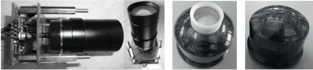
a) Long-range PIR hybrid sensor b) Close range PIR sensor c) Radar sensor
