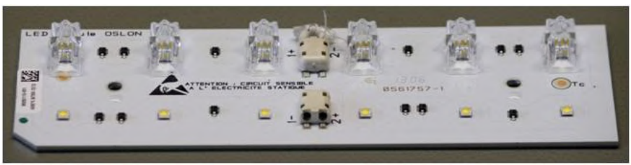
Fig. 2.20. LED3 luminary 28 W PCB plate module, voltage is 40 V DC and current is 700 mA.
