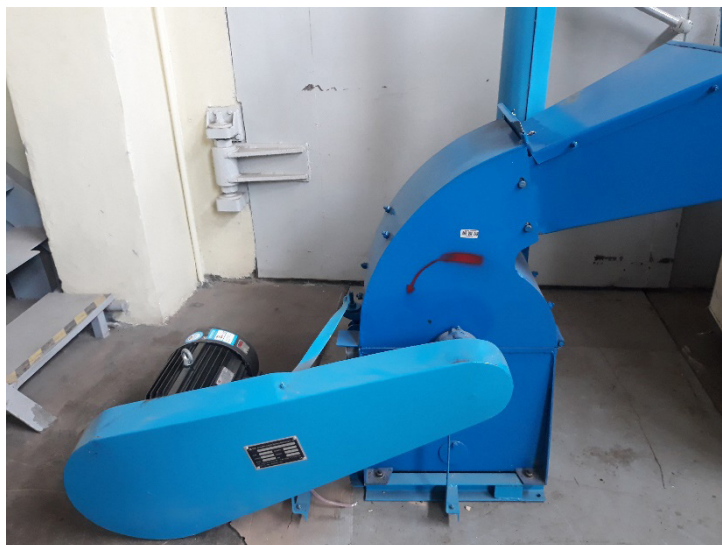
Figure 1. Installation of impact grinding of cadmium batteries with magnetic separation.
