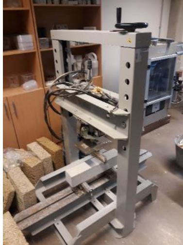
Figure 1. Testing process for concrete blocks with titanium reinforcement.
