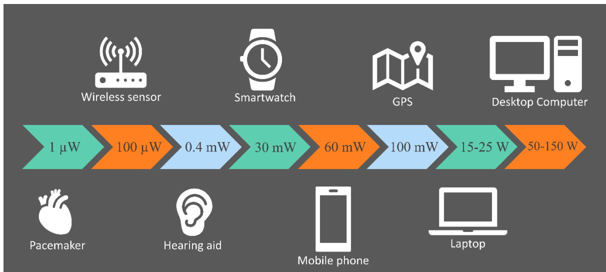
Fig. 1. Common electrical devices and their approximate power consumption.
