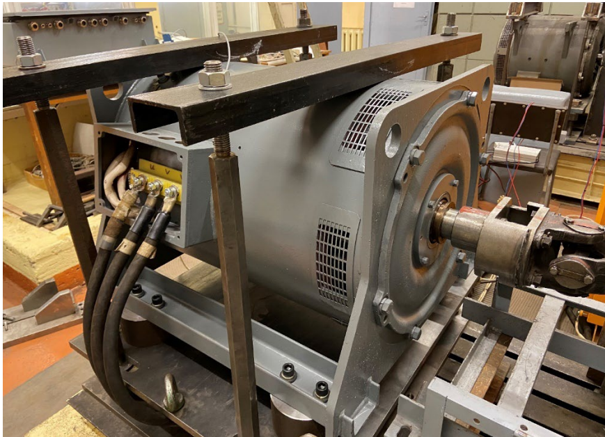
Fig. 4.2. SynRM traction drive on a test-bench.
