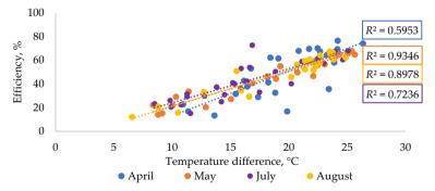
Fig. 2.8. Dependency of solar collector efficiency on the temperature difference.
