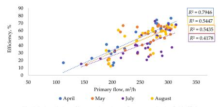
Fig. 2.7. Correlation of heat carrier primary flow rate and solar field efficiency.
