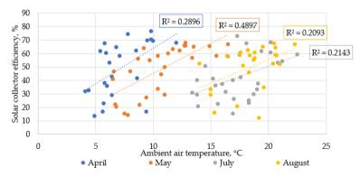
Fig. 2.9. Solar collector efficiency dependency on ambient air temperature.
