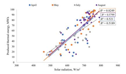
Fig. 2.3. Dependency of the produced solar energy on solar radiation.
