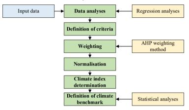
Fig. 1.1. Main steps and methods for determination of climate benchmark.
