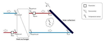
Fig. 2. Technical scheme of the measurement points [15].
