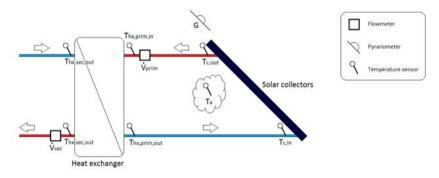
Fig. 2.7. Technical scheme of the measurement points [89]
