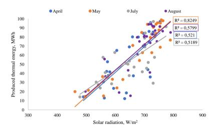
Fig. 3.8. Produced solar energy dependency of solar radiation
