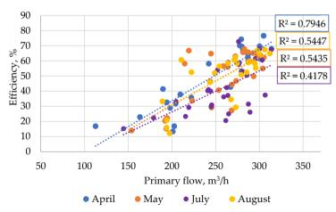
Figure 5. Correlation of heat carries primary flow rate and solar field efficiency.
