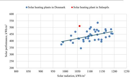
Fig. 6. Comparison of solar heating plant performance demanding of solar radiation in Denmark [13] and solar heating plant installed in Salaspils (2020).
