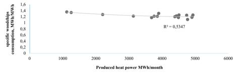
Fig. 2. Woodchips boiler specific woodchips consumption depending on produced heat power.
