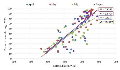
Fig. 4. Produced solar energy dependency of solar radiation.
