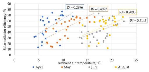
Figure 7. Solar collector efficiency dependency on ambient air temperature.
