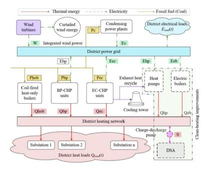
Fig.1.8. Schematic ilustration of a typical district energy system in China whith the cleanheating improvements [63]
