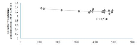
Fig. 3.3. Woodchips boiler specific woodchips consumption depending on produced heat power.
