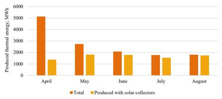
Fig. 3. Share of thermal energy produced by solar collectors and total produced thermal energy in 2019.
