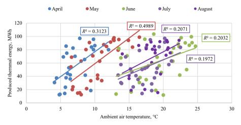
Fig. 5. Solar collector efficiency dependency of ambient air temperature.
