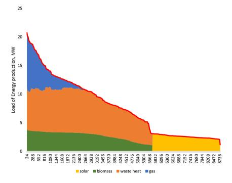
Fig.1.1. Heat load duration curve.
