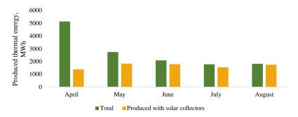
Fig.3.7. Share of thermal energy produced by solar collectors and total produced thermal energy in 2019
