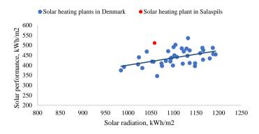
Fig.3.9. Comparison of solar heating plant performance demanding of solar radiation in Denmark (average data of 2012-2016) [94] and solar heating plant installed in Salaspils (2020)
