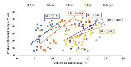
Fig. 3.9. Solar collector efficiency dependency of ambient air temperature
