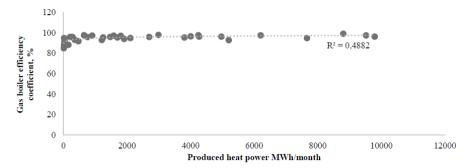
Fig. 3.4. Gas boiler efficiency coefficient depending on produced heat power
