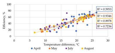
Figure 6. Solar collector efficiency dependency on temperature difference.
