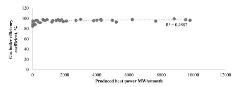
Fig. 3. Gas boiler efficiency coefficient depending on produced heat power.
