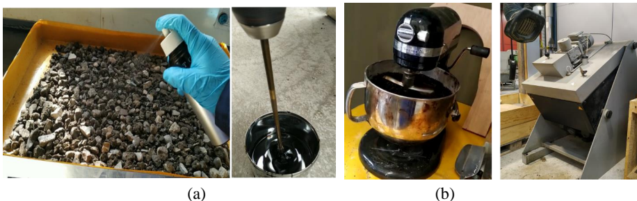
Figure 4.3. Laboratory mixing process (a) Spraying of rejuvenator on RA (left); Blending rejuvenator into the virgin binder (right), and (b) Small mixer (left) and Large mixer (right) used in the study
