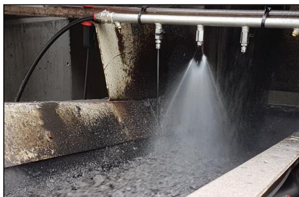
Figure 2.5. Spraying system for rejuvenator application on conveyor belt 19 (Vansteenkiste & Duerinckx, 2017)
