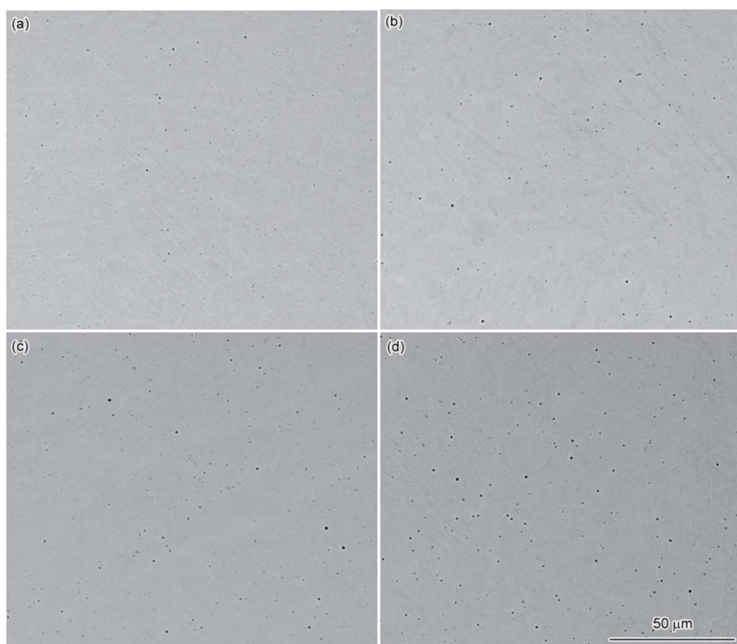
Fig. 1.18. Images of inclusions in the deposited metal with different shielding gases: (a) 95%Ar+5%CO 2 (b) 90%Ar+10%CO 2 (c) 80%Ar+20%CO 2 (d) 70%Ar+30%CO 2 [42].
