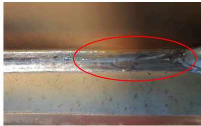
Fig. 2.7. Phenomena of SiO 2 on the welding seam.
