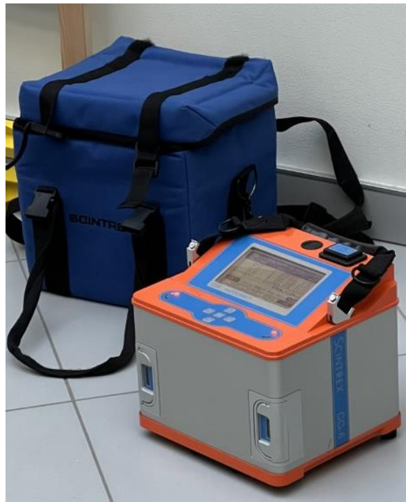
Figure 3.4. Scintrex CG-6 relative gravimeter ( author )
