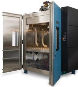
Fig. 4.8. VTC-36 stress screening or highly accelerated life testing chamber manufactured by CONTROLTECNICA [108].
