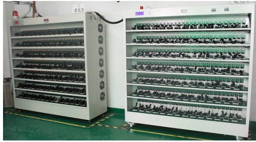
Fig. 4.25. Equipment of consumer grade power supply burn-in testing [165].
