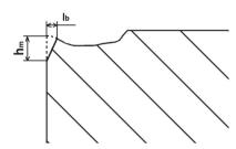
Fig. 16. Parameters of wear height h<sub>m</sub> and wear length l<sub>b</sub> on the insert in the cutting-edge slot.
