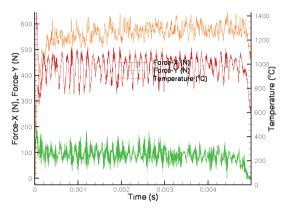
Figure 10. Cutting force and temperature values are a representation of the second simulation case [image by author].
