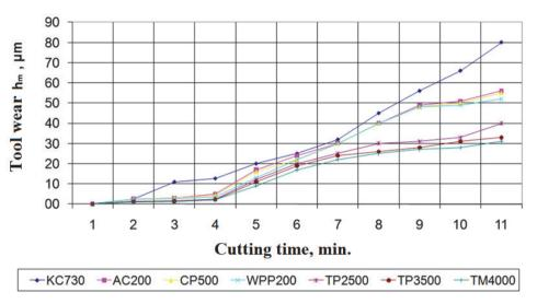
Fig. 20. Experimentally obtained results of tool wear.
