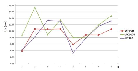
Fig. 13. AISI 420 graphic representation of average roughness values of the surface of stainless steel turned with tools of different materials.
