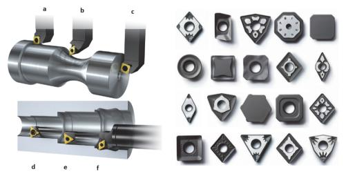
Fig. 1. Types of cutting operations in lathe [20].
