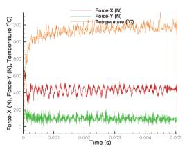
Fig. 9. The cutting force and temperature values are a representation of the first simulation case [developed by author].
