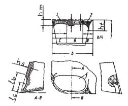
Fig. 14. Cutting edge wear parameters and designations, where: C, B, N – wear areas;  $l_b$  – length of wear hole;  $l_c$  – distance to the center of the wear hole;  $h_s$  – depth of the wear hole;  $h_m$  – flank wear;  $h_t$  – shock load wear; f – dimple wear form. [19].
