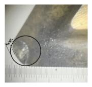
Fig. 19. Changes in the radius of rounding  $\Delta r$  on the wafer surface.
