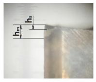
Fig. 17. Parameters of wear height h<sub>m</sub> and wear dent length h<sub>s</sub>.
