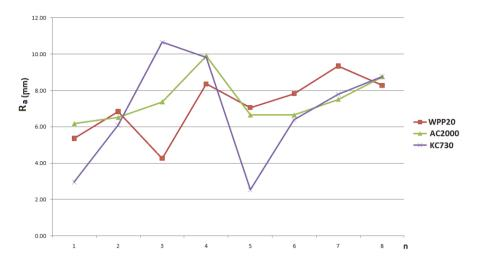
Fig. 12. AISI 304 graphic representation of the average roughness values of the surface of stainless steel turned with tools of different materials.
