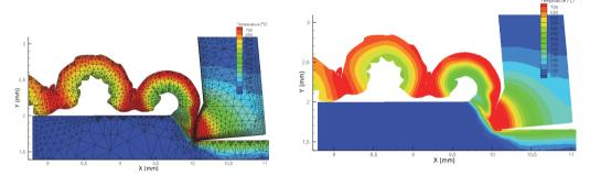
Fig. 5. General view of chip formation process and heat distribution field
