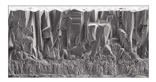
Fig. 4. Cutting tool coated with Duratomic technology, the vertical crystal positioning structure of the Al<sub>2</sub>O<sub>3</sub> coating is visible [22].
