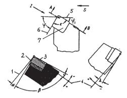
Fig. 15. Angles characterizing the cutting blade geometry , where: L – plane of the cutting edge of the tool; 2 – flank; 3 – chip surface; 4 – plane parallel to the basic plane of the tool; 5 – working plane; 6 – main cutting-edge setting plane; 7 – quick-changeable cutting insert;  $\alpha$  – back angle;  $\beta$  – wedge angle;  $\varphi$  – main setting angle;  $\varepsilon$  – apex angle;  $\lambda$  – inclination angle of the main cutting blade;  $\varphi$ 1 – auxiliary setting angle.[21].
