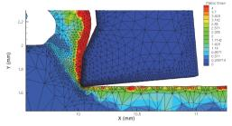
Fig. 7. Modeled distribution of contact stresses during the cutting process.
