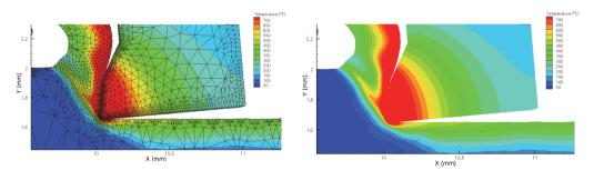
Fig. 6. The heat distribution field modeled during the cutting process in the enlarged scale with and without meshing.
