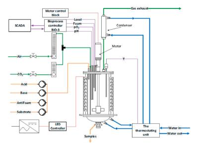
Fig. 1. The schematic diagram of sequencing batch photobioreactor for microalgae cultivation and synthetic wastewater treatment (© Bioreactors.net).
