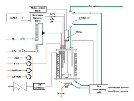
Figure 2.5. The schematic diagram of sequencing batch photobioreactor for microalgae cultivation and synthetic wastewater treatment (Copyright: Bioreactors.net).
