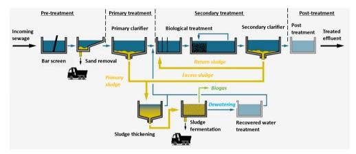
Figure 1.3. Conventional wastewater treatment plant scheme (Copyright: Jules van Lier, TU Delft)
