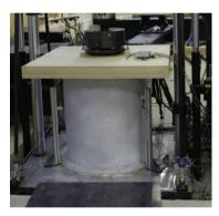
FIGURE 5: Experimental test setup for compressive loading on SST-2 cylindrical shell (RTU).
