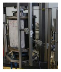
FIGURE 4: Experimental test setup for compressive loading on RI5 and SST-1 cylindrical shells (RTU).
