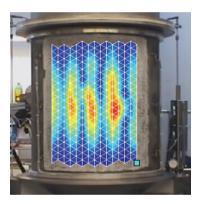
FIGURE 7: Fist vibration mode shape measured during testing (DLR-Z37).
