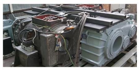
Fig. 5.16. Physical testbench of MGU under the mutual load control.
