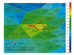
Fig. 4.5 Maximal main stresses at point "1" for Mode III.
