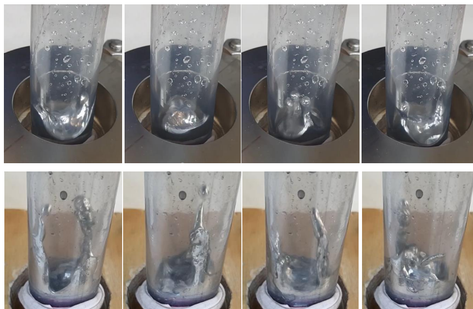
Fig. 4.10. InGaSn free surface electromagnetic stabilization experiment at 20 Hz: a) with applied magnetic field (above); b) – without magnetic field (bottom).
