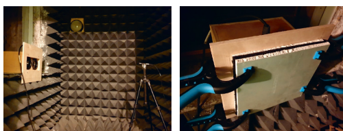
Semi anechoic chamber and insertion loss measurement stand.
