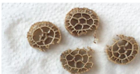
Figure 1. Mechanically damaged K3 biofilm carriers from denitrification process.
