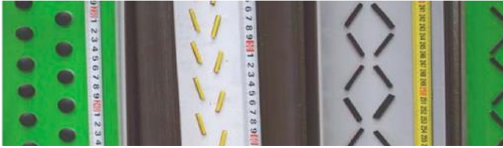
Figure 1. Samples of surfaces with artificial roughness used during the experiments. Left to right: round obstacles; cylindrical bars; cruciform bars arranged in the form of a parallelepiped; the same with a round obstacle in the middle; corners and double obstacles in the form of wedges.
