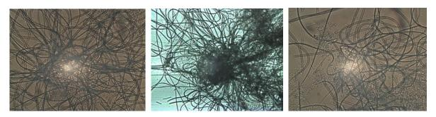
Fig. 5. P deficiency-induced dominance of filamentous bacteria in GWWTP activated sludge (magnification 100 x, light microscope Optika B-600 Tiph).
