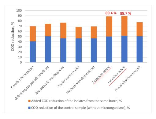
Fig. 4. Efficiency of COD reduction using bioaugmentation with yeast and filamentous fungal cultures.
