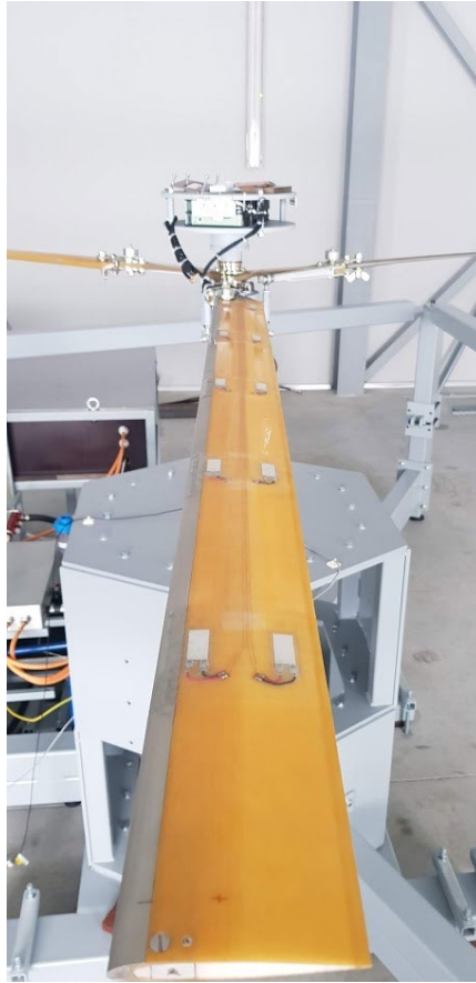
Fig. 4.5. Blade with piezo film sensors and measurement system.
