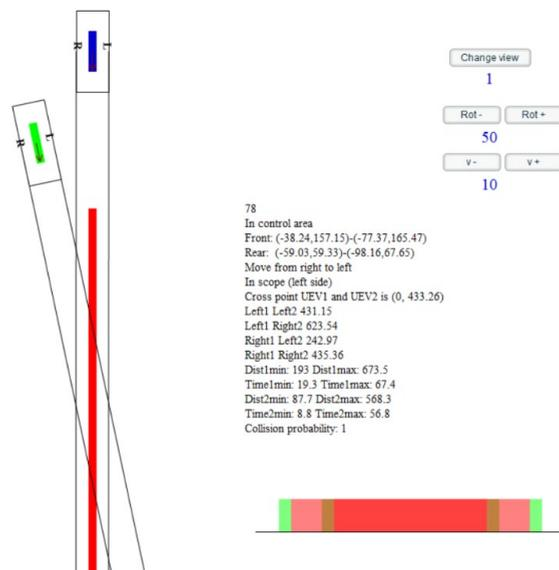
Fig. 5.1. Testing of the algorithm of collision probability evaluation of UEVs.
