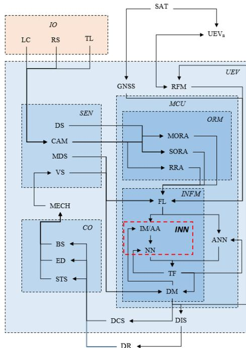
Fig. 1.1. Scheme of the distributed system structure with reduced number of components.
