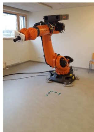
Fig. 2. Industrial robot manipulator of 210 g payload class representing basis for typical industrial manufacturing related research tasks.
