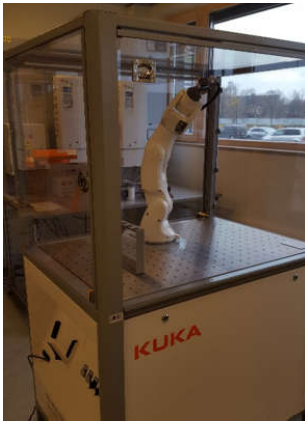
Fig. 3. KUKA small scale industrial robot manipulator for teaching and programming concept evaluation tasks.
