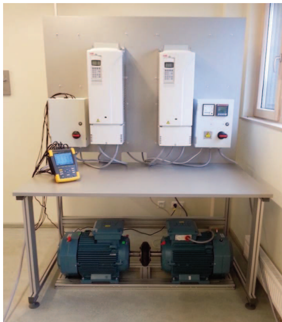
Fig. 2. Laboratory test bench setup of the motor drive system. FC1 and M1 are located on the left side and FC2, M2 on the right side with their respective power supply enclosures.
