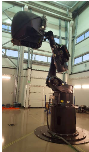
Fig. 1. Large motion range physical simulator based on KUKA KR 600 series industrial robot manipulator.
