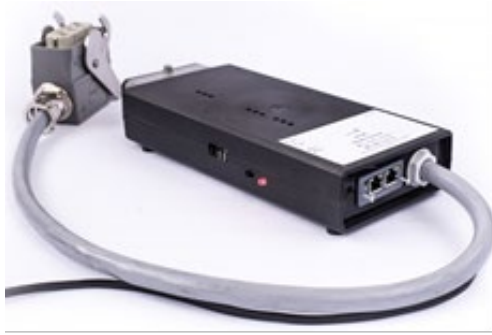
Fig. 3.19. Power flow meter as industrial robot extension cable.
