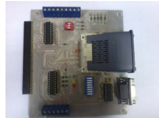
Fig. 5 Communications and IGBT control module.
