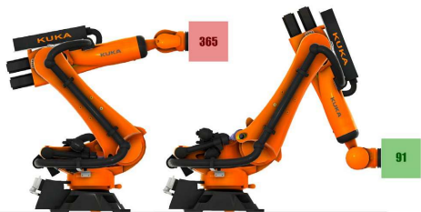
Fig. 4. Most efficient and most inefficient robot configurations according to energy map.
