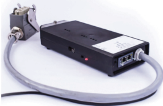
Fig. 6. Bi-directional AC/DC power / energy flow meter; 20 ms energy sampling rate.
