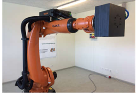
Fig. 4. Industrial robot manipulator equipped for toll mass variation related experiment.
