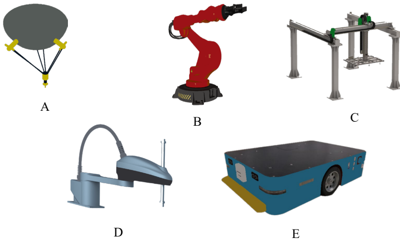
Fig. 1.1. Industrial robot types: A) – Delta; B) – articulated manipulator; C) – Cartesian (linear); D) – SCARA-type; E) – autonomous guided vehicle (AGV).
