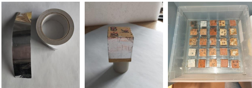
Figure 5.. From left. Tape, sample prepared, partial immersion
