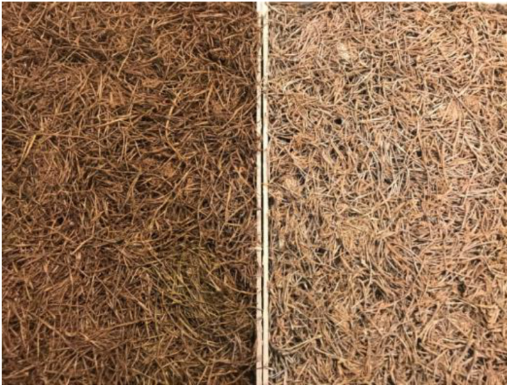
Fig. 2. Pine needle insulation material sample without lime (on the left) and with lime (on the right).
