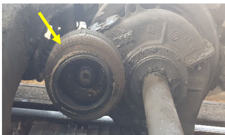
Fig. 1.3. Example of rubber-cord coupling layer rupture.
