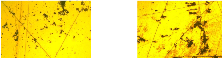
Fig. 3.37. Metallographic analysis of bolt Sample 26, mileage 79 906 km.
