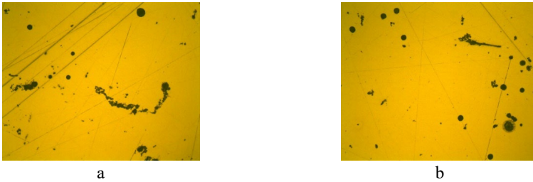
Fig. 3.32. Metallographic analysis after 360 impacts with a force of 20 000 N, magnification – \times 200 :
