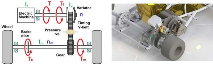
The drive of the go-kart. (A) Schematic of the CVT dynamic model; (B) 3D model of the CVT on the go-kart.
