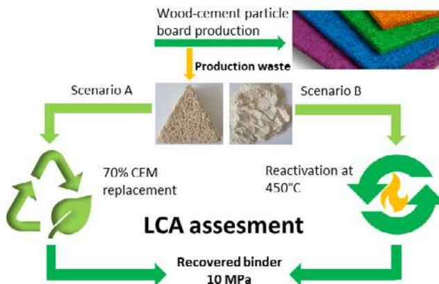
LCA scenarios of wood-cement particle board production waste recovery.
