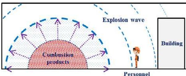
The scheme of the blast wave propagation in the area of the accident.
