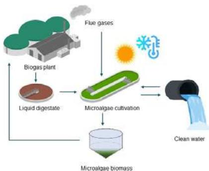
Nutrient removal from agricultural digestate by integrating microalgae cultivation into a biogas plant offers a closed-loop circular economy perspective also in low-temperature regions.
