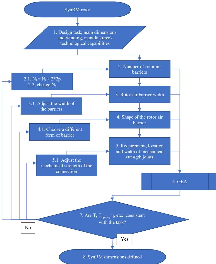
Fig. 2.6. SynRM rotor sizing algorithm.
