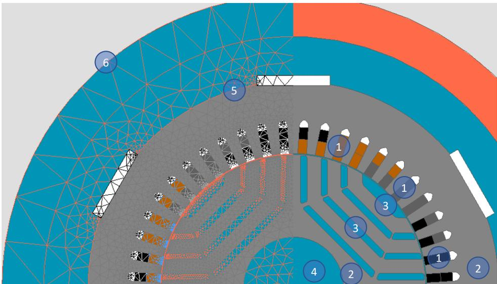
Fig. 2.15. SynRM FEM model with finite element mesh.
