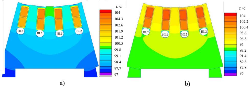
Fig. 3.6. FEM simulation results for a SynRM segment with HL2 in the stator slots:
