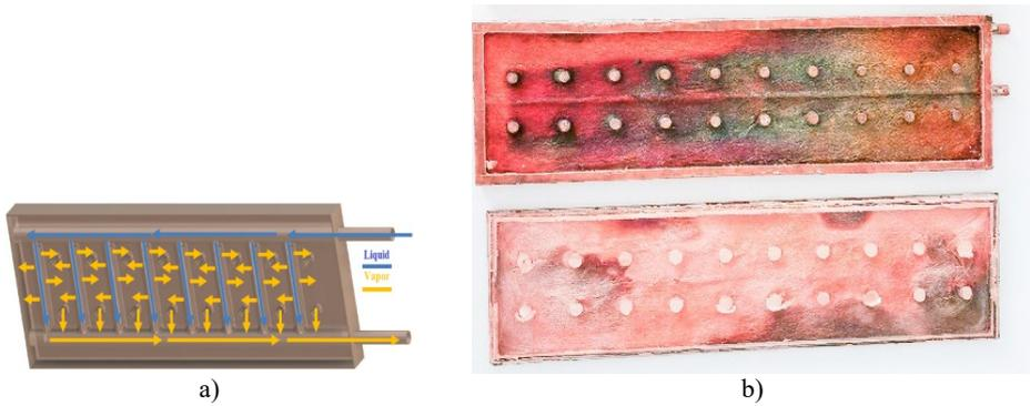
Fig. 4.10. HL evaporator: a) schematic representation; b) fabricated capillary effect evaporator with wick-shaped copper parts.
