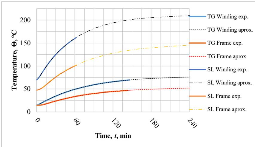
Fig. 4.19. SynRM with HL winding and case heating in no-load (TG) and load (SL) modes.
