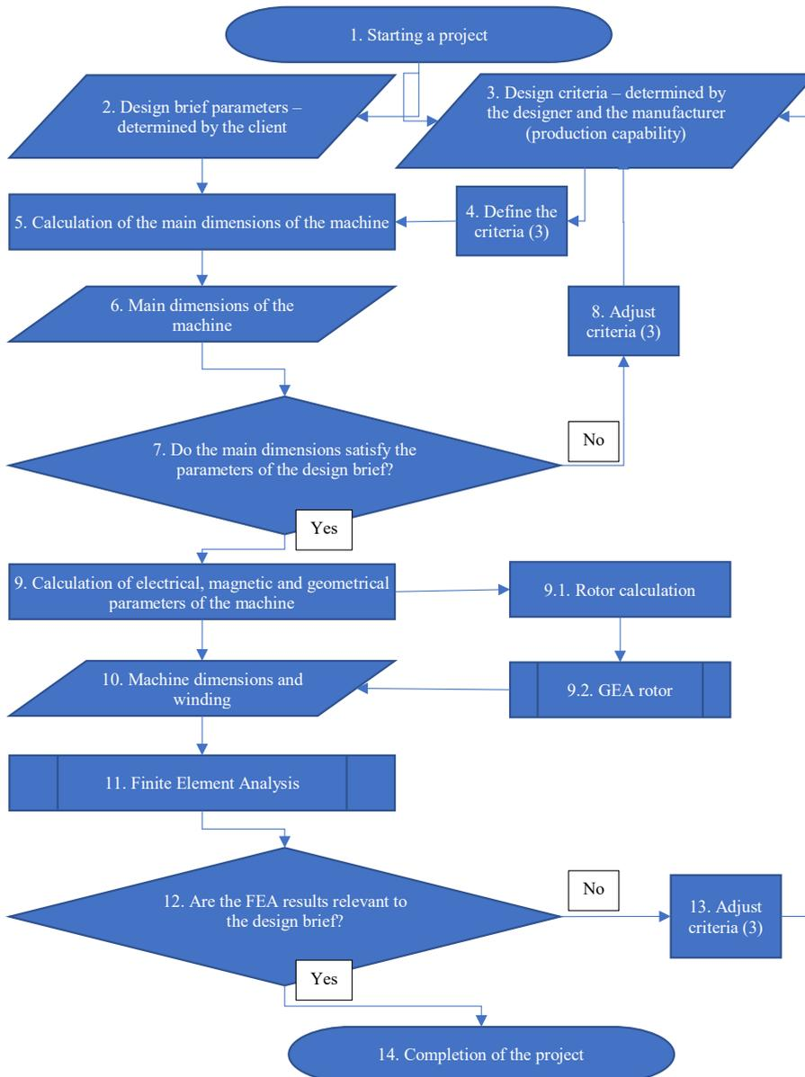
Fig. 2.3. SynRM design flow chart.
