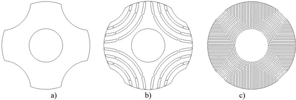
Fig. 2.4. SynRM rotor designs: a) salient pole; b) non-magnetic air barrier; c) axially laminated electrical steel sheets.
