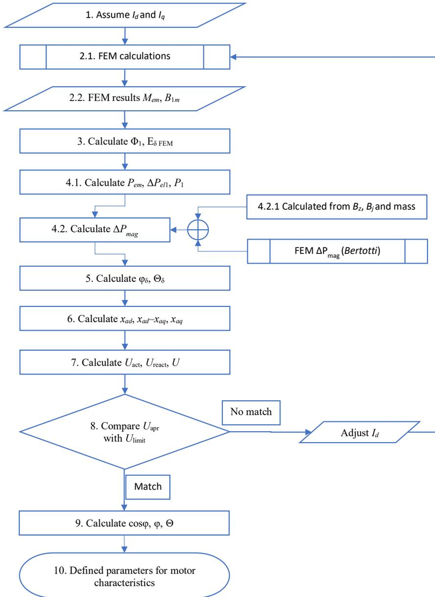
Fig. 2.14. Sequence of steps in the algorithm for calculating characteristic curves.
