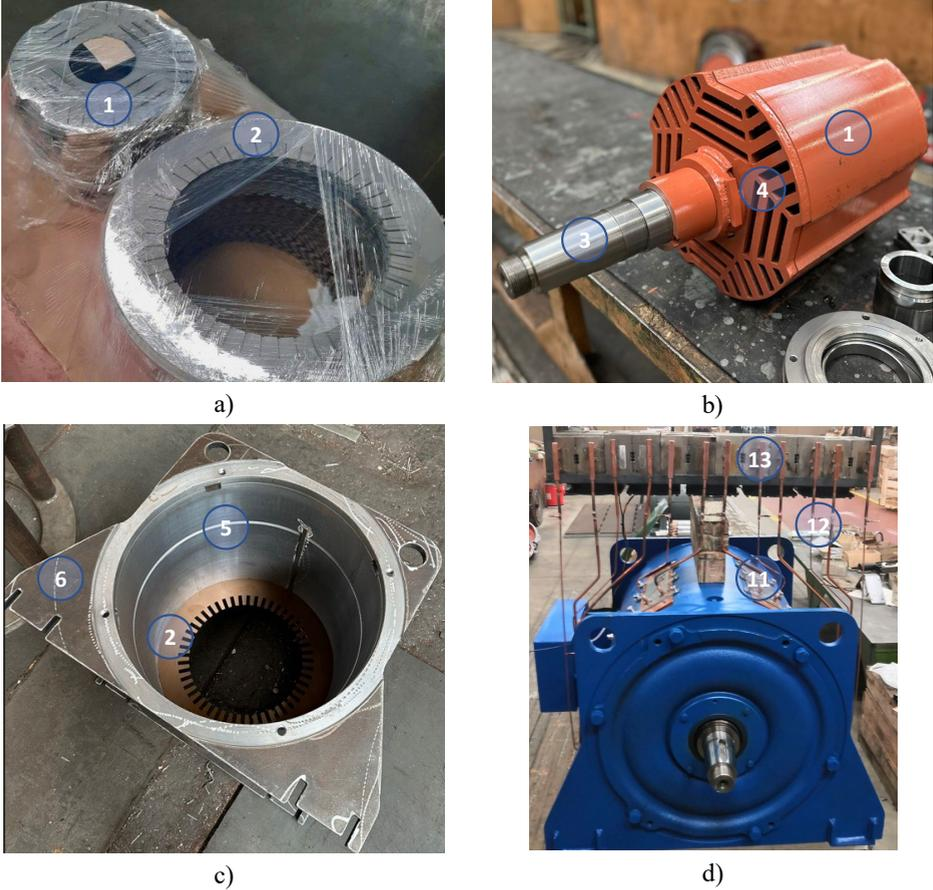
Fig. 4.15. Process for making SynRM with HL.
