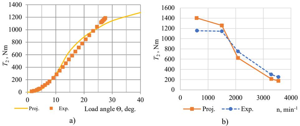
Fig. 4.7. 180 kW SynRM experimental and calculated performance curves: a) static, angle characteristic; b) traction characteristic.
