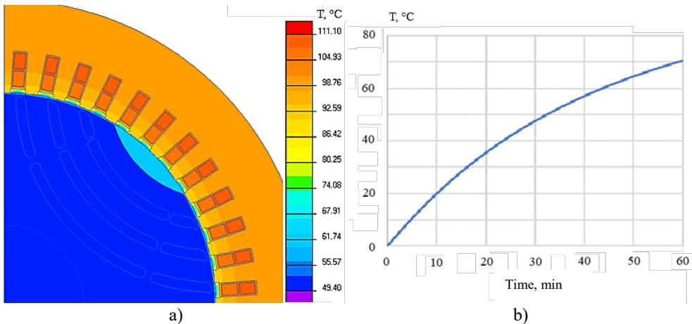
Fig. 3.4. FEM simulation results for 180 kW SynRM: a) temperature distribution in the machine, steady state; b) temperature variation in the stator slot or winding with operating time, summary of FEM results.
