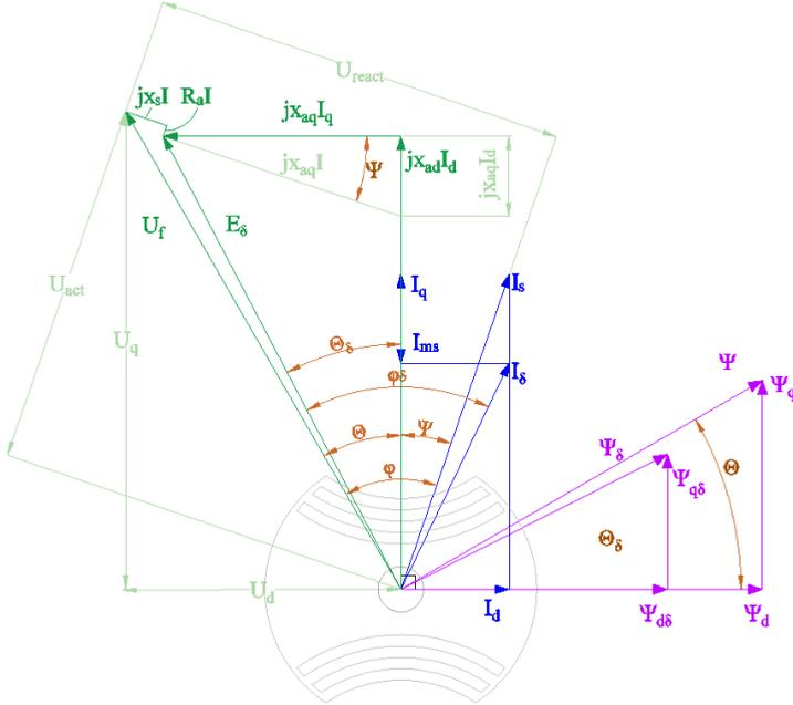
Fig. 2.13. 180 kW SynRM vector diagram,  $I_N = 372\text{A}$ ,  $U_N = 420\text{V}$ , nominal load mode.
