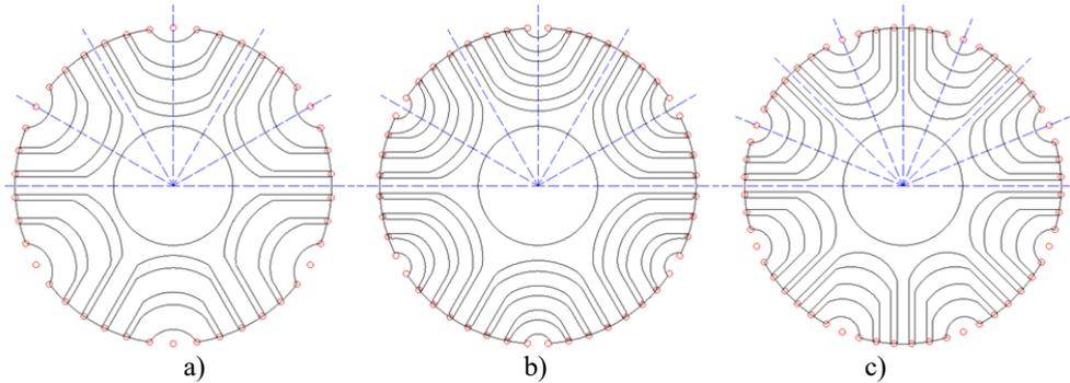
Fig. 2.5. SynRM design with different numbers of poles and rotor air barriers: a)  $2p = 6$ ,  $N_r = 42$ ; b)  $2p = 6$ ,  $N_r = 48$ ; c)  $2p = 8$ ,  $N_r = 56$ .
