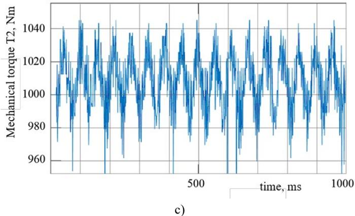
Fig. 4.8. 180 kW SynRM experimental and calculated curves: a) stator winding temperature  $\Theta_w$ ; b) electromagnetic torque ripple, instantaneous value from FEM calculations; c) mechanical torque ripple, from experimental results.
