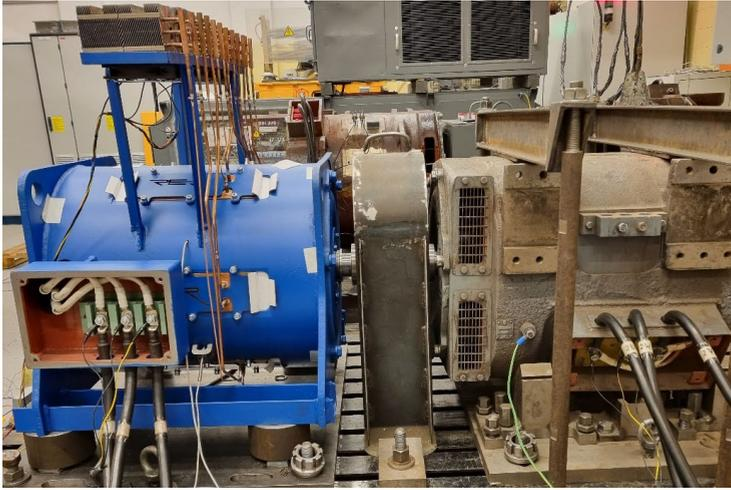
Fig. 4.16. SynRM with HL experimental bench.
