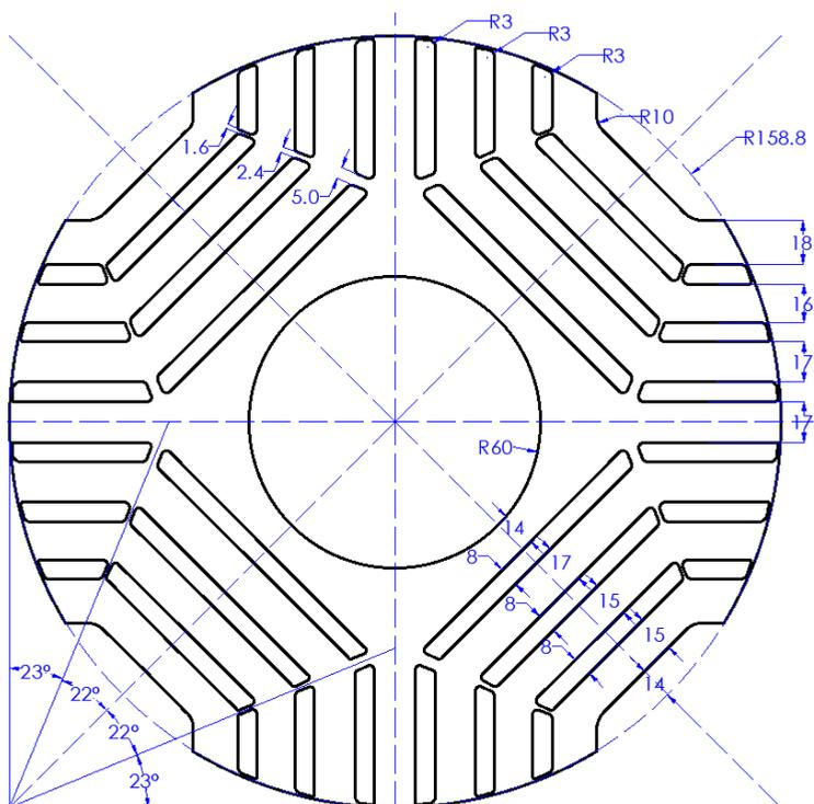
Fig. 4.14. SynRM with HL cooling, trapezoidal air barrier rotor.
