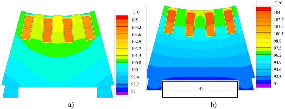
Fig. 3.5. FEM simulation results for the SynRM segment:
