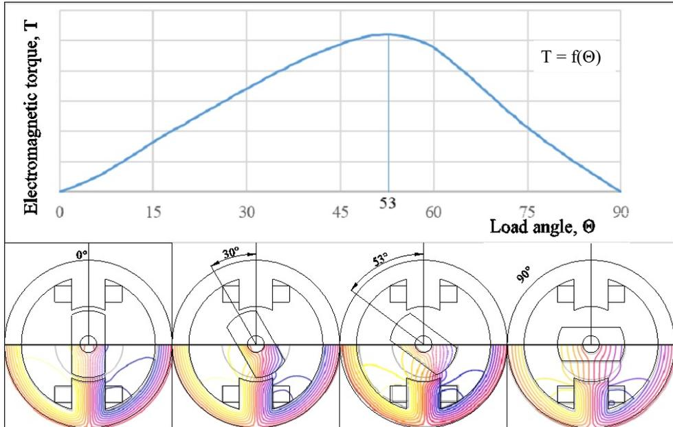
Fig. 2.2. Electromagnetic torque versus load angle.
