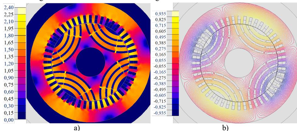
Fig. 4.1. Magnetic field in nominal mode:  $I = 392$  A,  $I_d = 125$  A,  $I_q = 372$  A;  $\Theta = 29.9^\circ$ :
