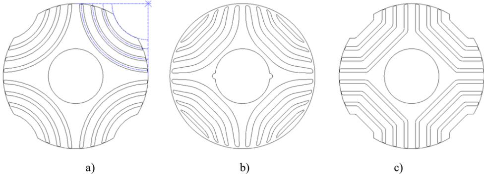
Fig. 2.9. Shape of air barriers: a) arch with common centre; b) trapezoidal with rounded corners; c) trapezoidal.
