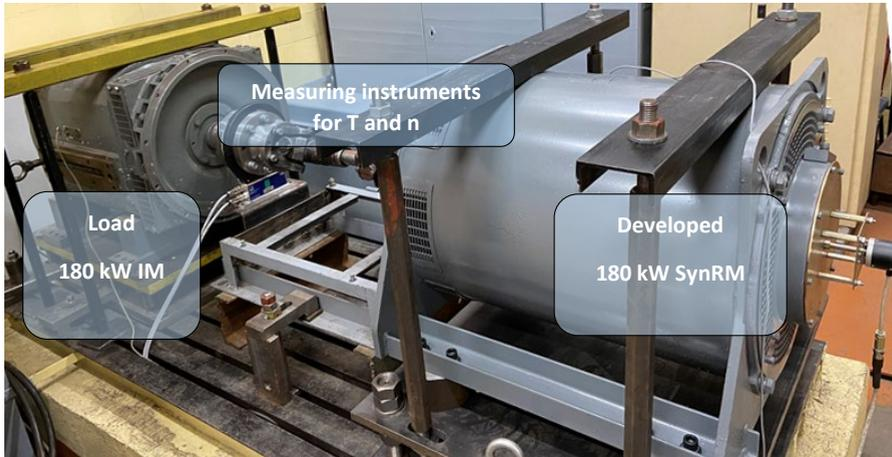
Fig. 4.5. 180 kW SynRM test stand.
