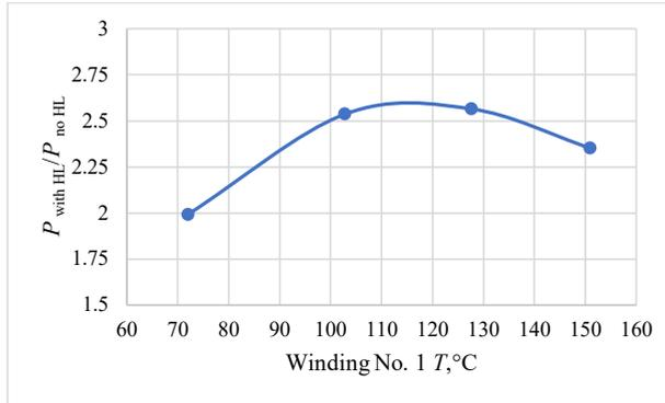
Fig. 4.11. Ratio of power applied to segment windings with and without HL cooling at steady-state temperature.
