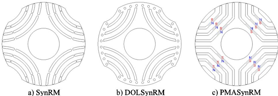
Fig. 2.1. Synchronous reluctance motor rotor designs:
