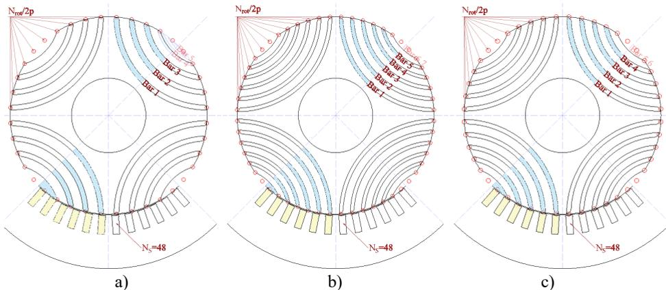
Fig. 2.7. Number of air barriers, SynRM with  $2p = 4$ ,  $N_s = 48$ :
