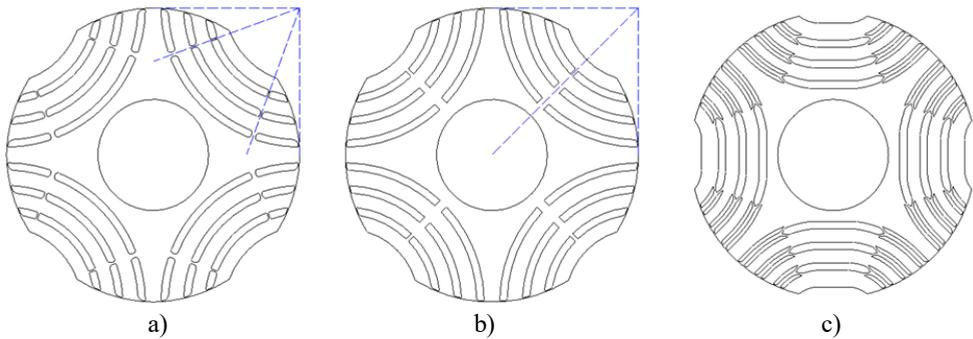
Fig. 2.11. Location and shape of mechanical strength connections: a) shifted from the q-axis; b) on the q-axis; c) connections with a complex shape.
