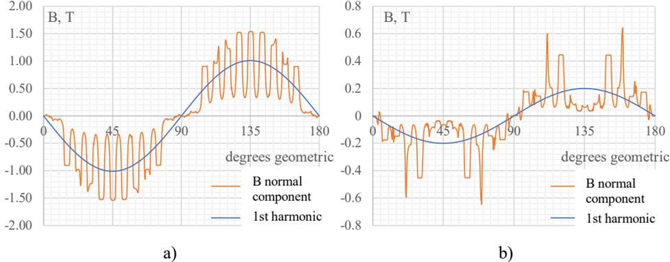
Fig. 4.3. Magnetic flux density in the air gap at no load, normal component: a) d-axis (d); b) q-axis (q).
