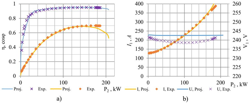
Fig. 4.6. 180 kW SynRM experimental and calculated performance curves: a) efficiency and power factors; b) voltage and current.
