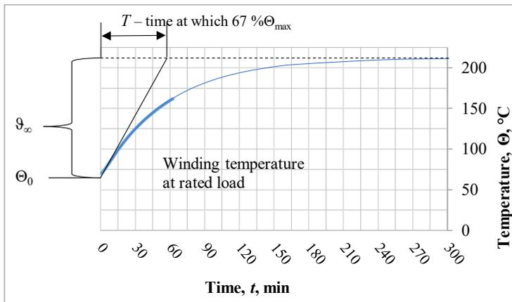
Fig. 4.18. SynRM with HL winding temperature  $\Theta_0$ ,  $\vartheta_{\infty}$  and heating time constant  $T$ .
