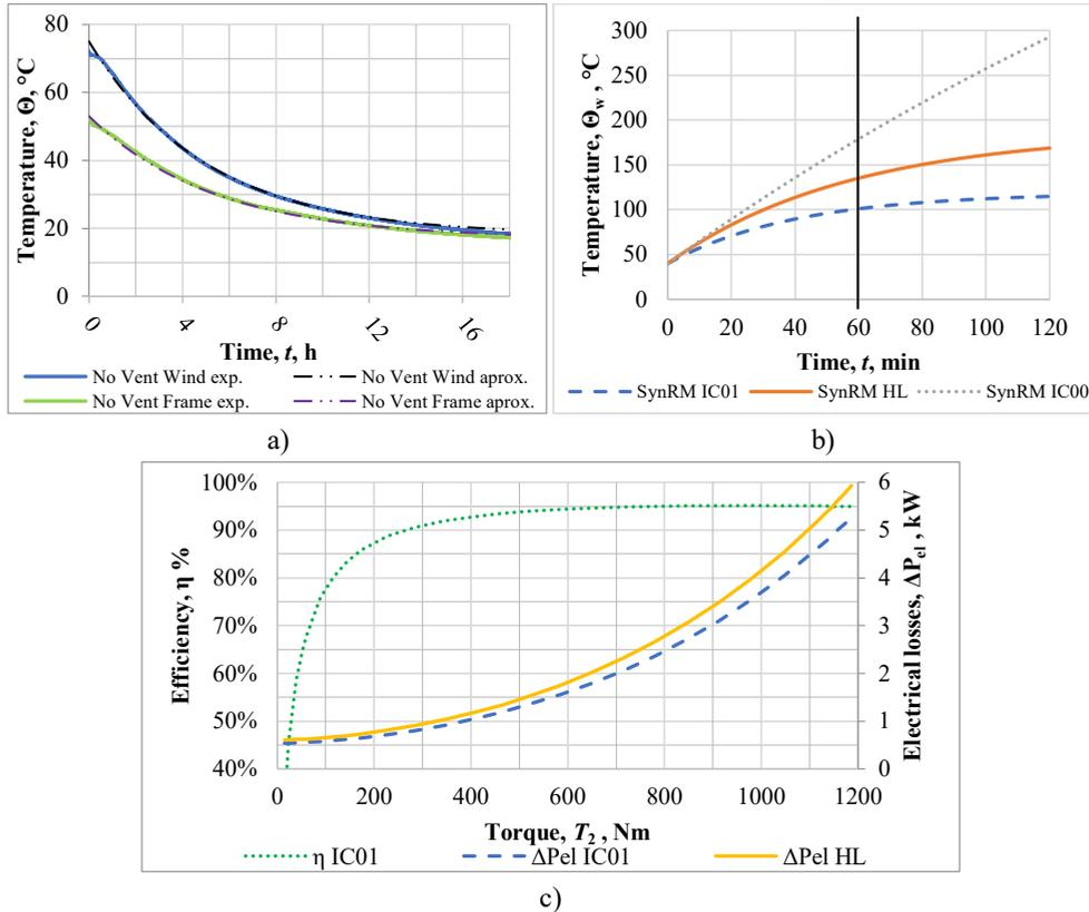
Fig. 4.20. a) SynRM with HL, winding (Wind) and frame (Frame) cooling experiment results (exp.) and calculated approximation (aprox.) with HL vapour condenser fans off (No Vent); b) SynRM with HL, SynRM IC01 and SynRM IC00 temperature comparison at ambient temperature,  $\Theta_{\text{amb}} = 40 \text{ }^\circ\text{C}$ ; c) Electrical losses of SynRM with HL and SynRM IC01 vs. load torque, at  $n = 1500 \text{ min}^{-1}$ ,  $U = 420 \text{ V}$ ,  $f = 50 \text{ Hz}$
