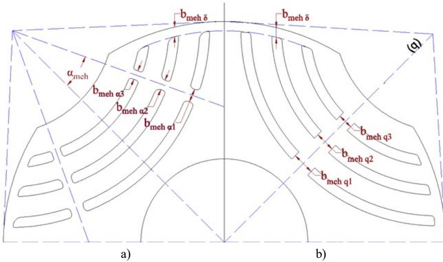
Fig. 2.10. Illustrative sketch of mechanical strength connections and their main dimensions: a) q-axis offset connection; b) q-axis connection.
