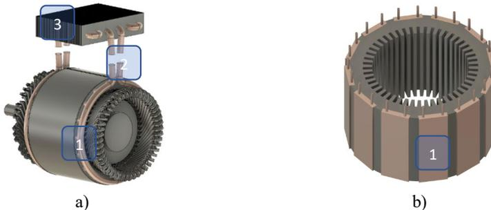
Fig. 3.3. Heat loops cooling system: a) main elements of the heat loops; b) stator design with 12 evaporators.
