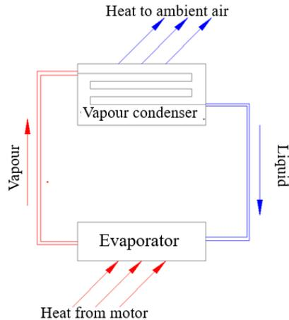
Fig. 3.2. Operating principle of a heat loop (HL).
