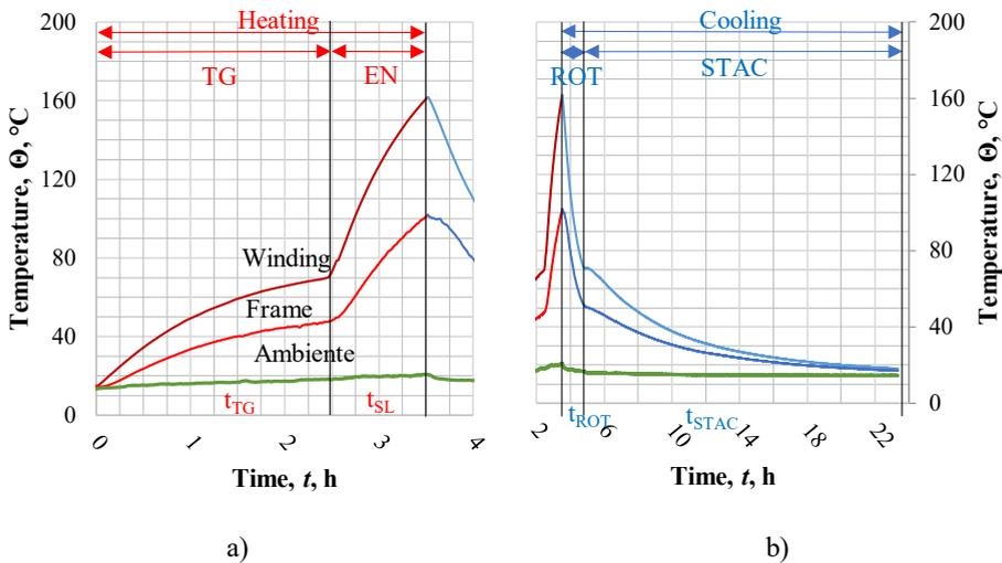
Fig. 4.17. Results of the SynRM with HL experiment: a) heating at no load (TG) and nominal load (SL) modes; b) cooling with HL evaporator fans on (ROT) and HL evaporator fans off (STAC).
