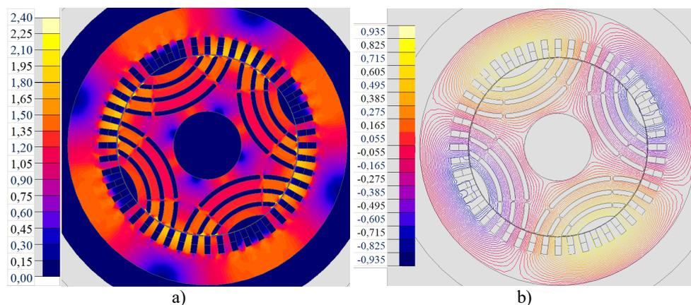
Fig. 4.2. Magnetic field at no load:  $I = 126$  A,  $I_d = 126$  A,  $I_q = 0$ ;  $\Theta = 0$ :
