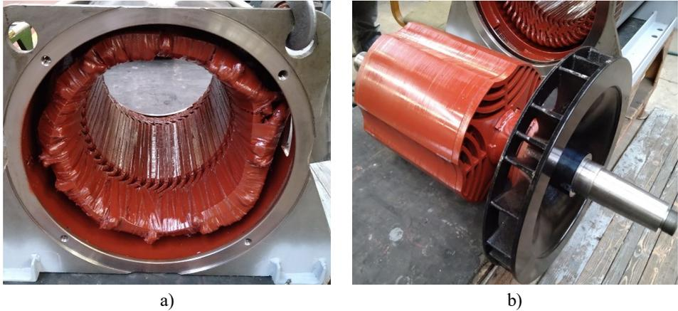
Fig. 4.4. 180 kW SynRM manufactured by JSC "RER": a) stator; b) rotor.
