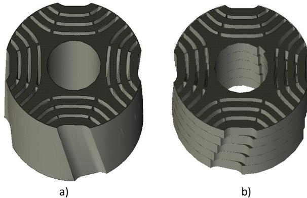
Fig. 2.12. SynRM with skewed rotor: a) skewing each sheet of electrical steel by a small angle; b) dividing the rotor into segments and skewing the segments.
