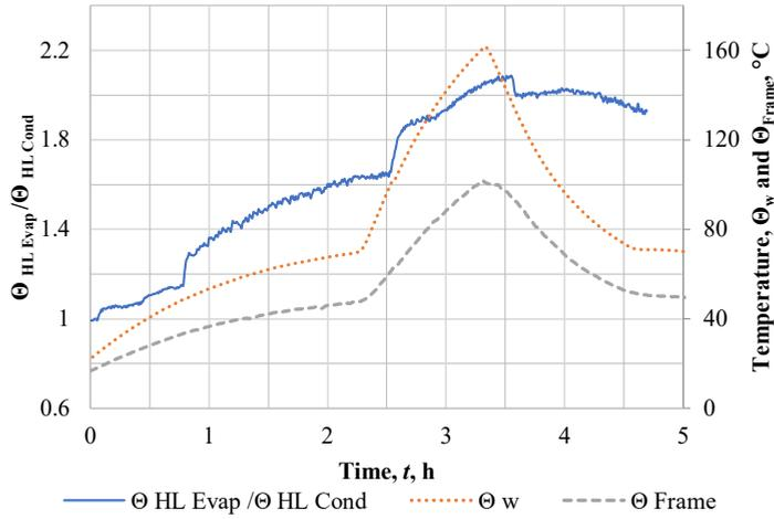
Fig. 4.22. Relationship of HL evaporator (HL Evap) and HL vapour condenser (HL Cond) temperatures on the same time scale with winding and frame temperatures.
