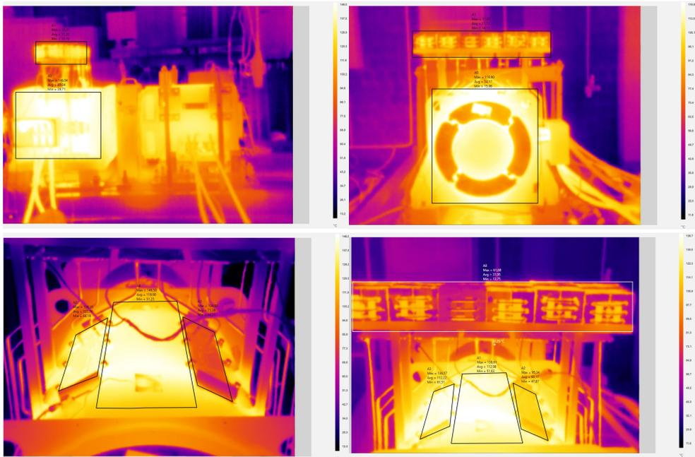
Fig. 4.21. Thermal images of the SynRM with HL before the cessation of the heating mode when the maximum motor temperatures are reached.
