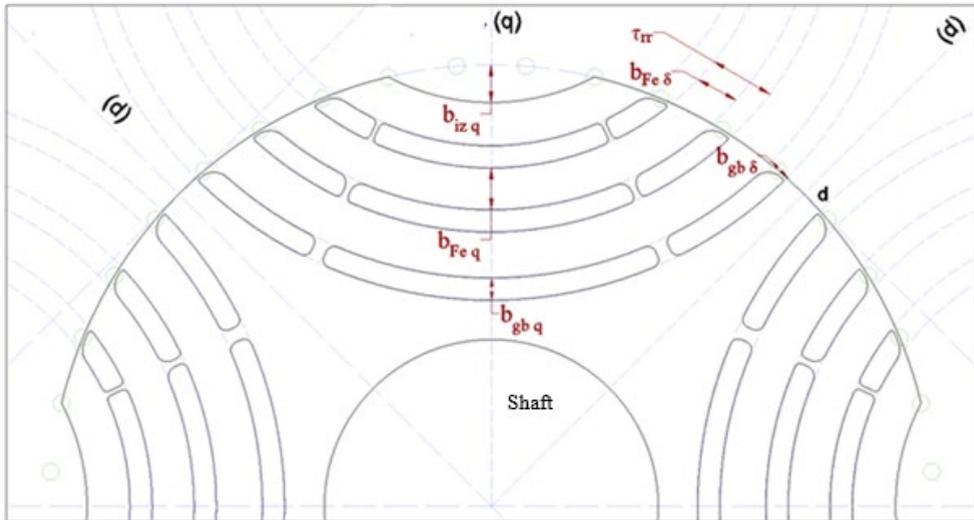
Fig. 2.8. Dimensions of rotor air barriers and flux channels.
