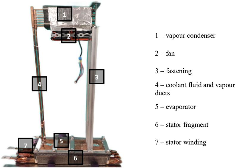
Fig.e 4.9. Stator segment with HL cooling.
