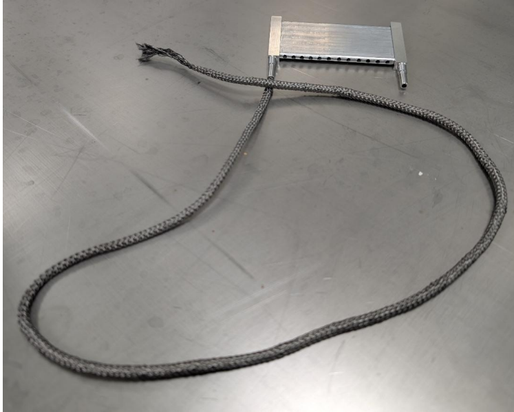
Figure 6-6. Evaporator with an extended wick, prepared for welding.
