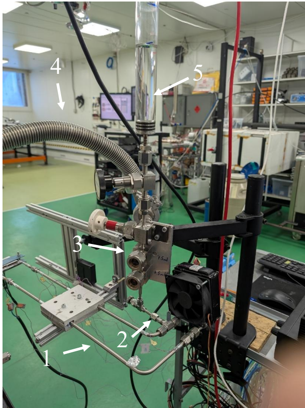
Figure 6-10. Loop Thermosyphon charging setup. 1) LTS; 2) Charging port; 3) Charging station; 4) Hose to vacuum stand; 5) Volume with toluene
