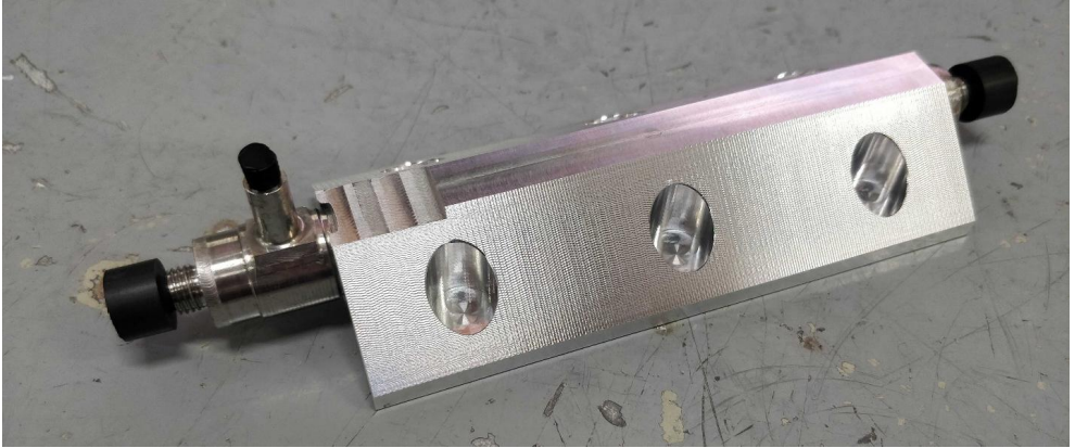
Figure 3-4. A saddle machined from a single piece of aluminium, with the capillary pump installed by vacuum brazing.
