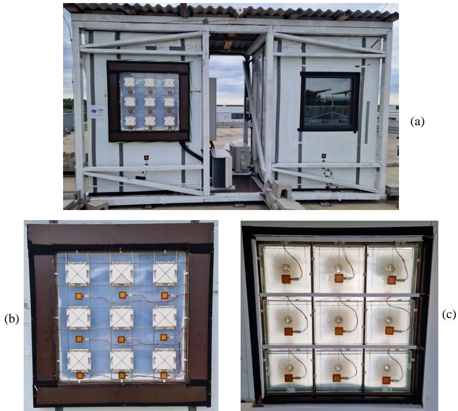
Fig. 3.9. Testing (left) and reference (right) stands (a); solar facade system containing nine small-scale dynamic modules from outside (b) and inside (c) testing booth.
