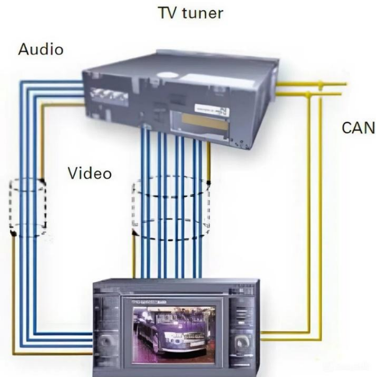
Fig. 3.19. Communication diagram of control units via the MOST bus [6].
