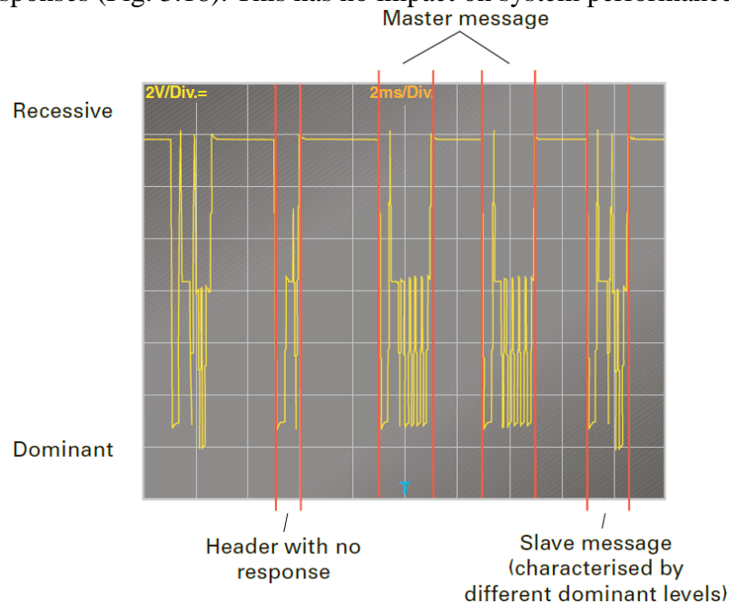
Fig. 3.18. Typical telegram structure [6].
