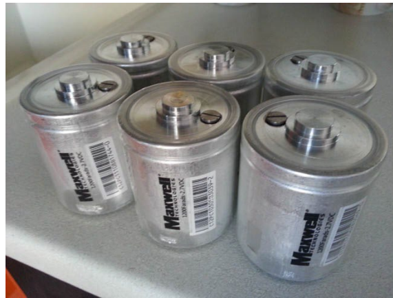
Figure 2.6. General view of supercondencers Maxwell 1200F, 2.7V
