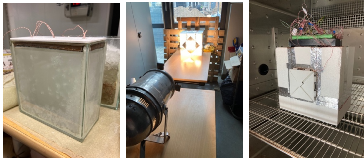
Fig. 4. PCM in solid state (left), heating phase (in the middle) and cooling phase (right).
