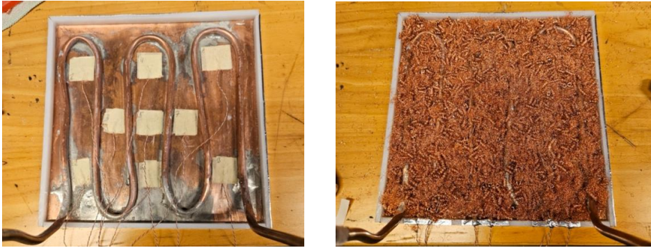
Fig. 3.2. Design of the hot/cold plate for the apparatus.
