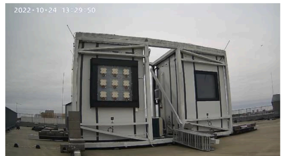
Fig. 16. Testing booths on the roof. Location – Riga, Latvia. Left solar façade module built in, right – reference booth with triple glazed window.
