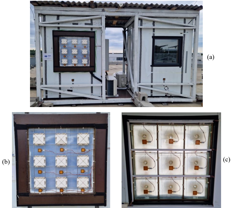
Fig. 5.6. Testing (left) and reference (right) stands (a); solar facade system containing 9 small-scale dynamic modules from outside (b) and inside (c) testing booth.
