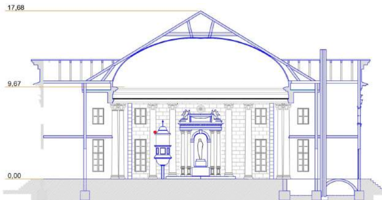
Fig. 9. Cross-section of the Riga Jesus Church with the installed measuring devices.
