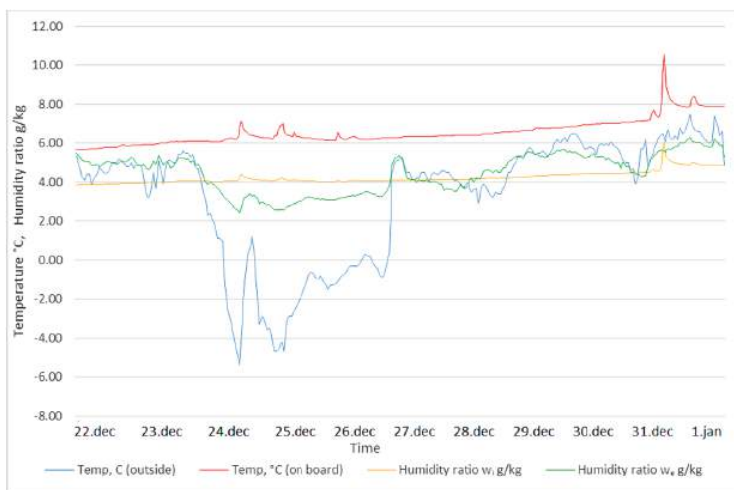
Fig. 15. Outdoor and inside moisture and temperature in Liepaja St. Trinity Cathedral on the board between 12/22/2022 and 01/02/2023.
