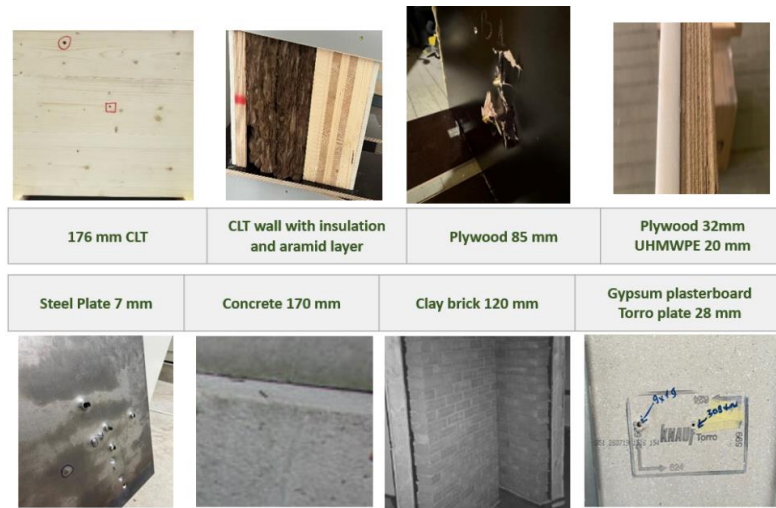
Fig. 5.7. Eight analysed ballistic wall systems, illustrated with representative images. [9], [20], [36], [41], [42], [43]
