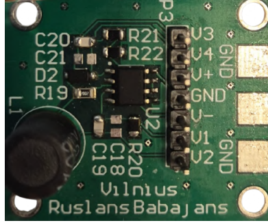
Fig. 1.5. Fabricated Vilnius chaotic oscillator PCB prototype.
