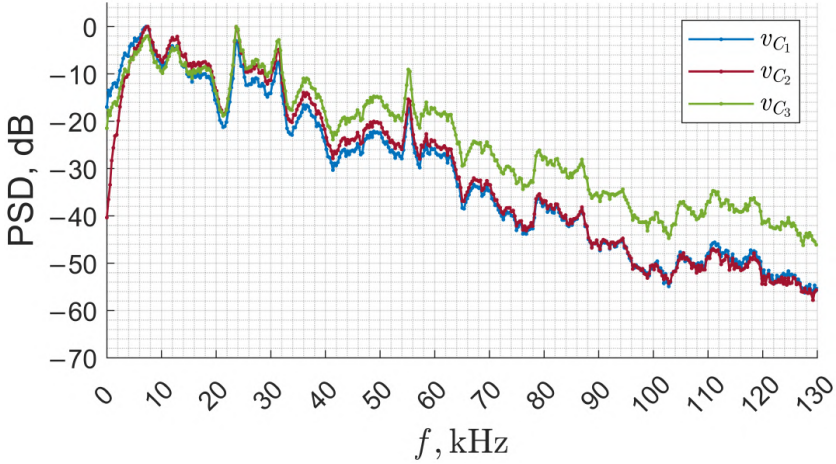
Fig. 1.14. PSD of v_{C_1} , v_{C_2} and v_{C_3} for the RC chaotic oscillator prototype.
